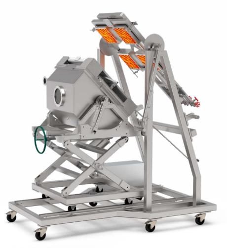
For the building industry, fire behavior including flammability and flame spread is of major importance. With the TDP T4 testing device, the behavior of roofs when exposed to external fire loads can be determined.
