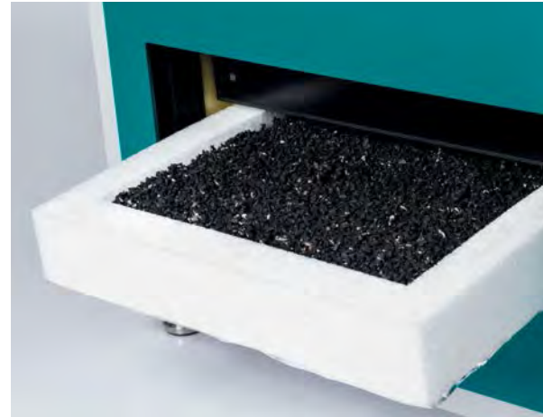
Measuring frame for loosely filled material
