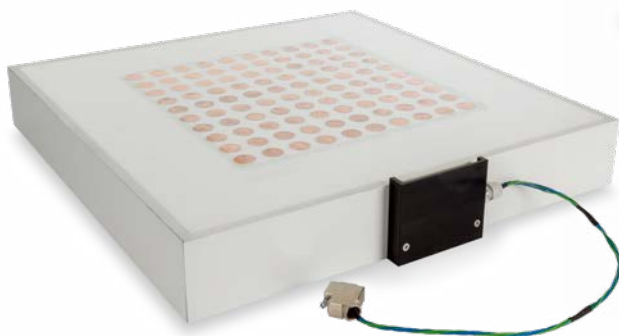
Specimen adapter plate for 1-specimen mode
